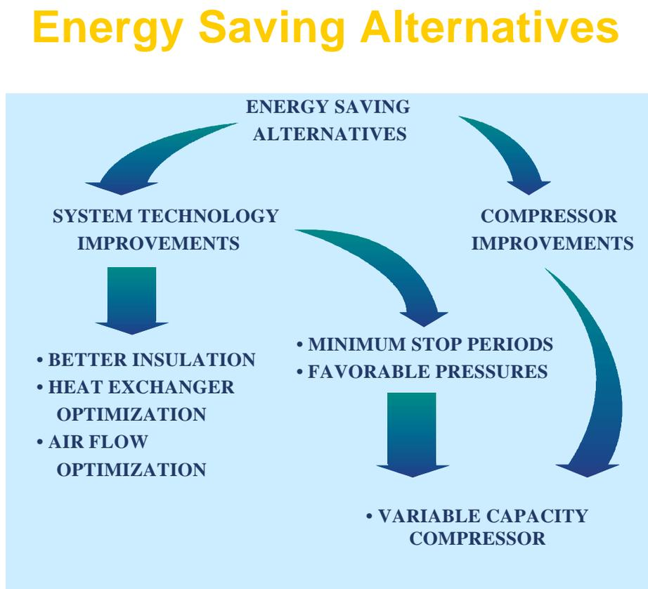
It is clear that thermal insulation, the intrinsic compressor COP (Coefficient of Performance-which expresses the compressor’s energy efficiency), and the thermodynamic behavior of the sealed system, are the basic areas with a fundamental effect on the appliance energy consumption, and can be worked independently to obtain benefits.
