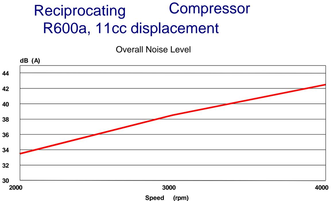
The Variable Capacity Compressor represents an excellent opportunity for a direct overall noise reduction in appliances, because it offers the possibility to operate most of time at speeds lower than 3000 or 3600 rpm.
