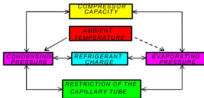
FIG 5 – Design Routine for Variable Capacity Compressor
